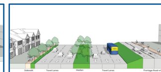
Mixed Traffic BRT Alternative 3C
